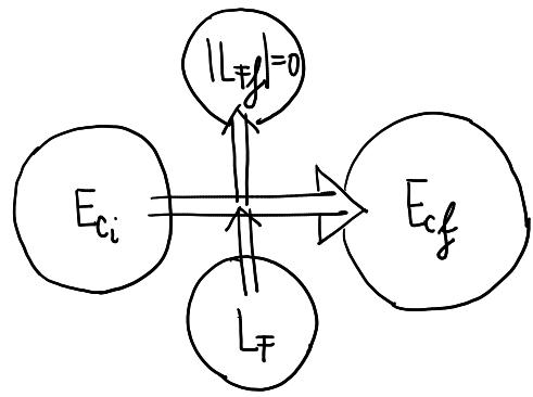
$$\begin{aligned} i \rightarrow f: \quad & E_{ci} + L_F - \cancel{|L_F|}^0 = E_{cf} \\ \Rightarrow \quad & E_{cf} - E_{ci} = L_F \end{aligned}$$
